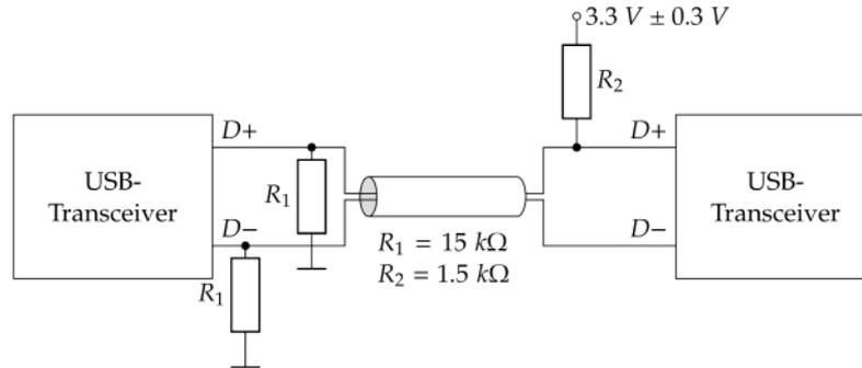
Figure 2.1: Example for resistor configuration at 12Mbit/s
