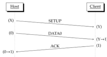
Figure 2.2: Synchronization of the data toggle sequence bits
